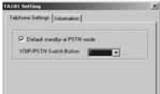
If the box for **Default standby at PSTN mode** is activated, outgoing calls are made via the existing analogue telephone line by default. To hold the conversion using VoIP, switch to VoIP using **“\*\*”** before dialling the number.
